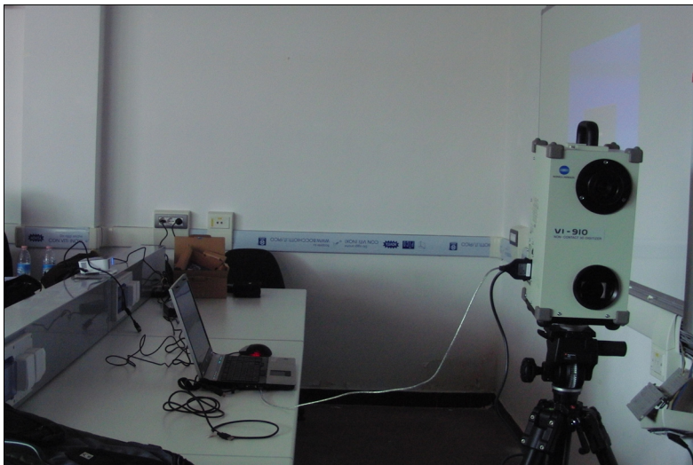
Hardware: laser scanner Vivid 910
