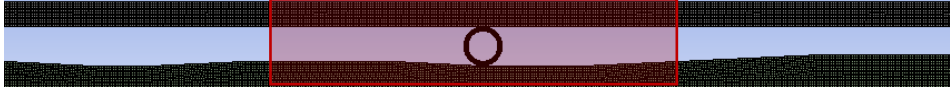
Fig. 5.16 – Undeformed geometry of the hollow MoS 2 nanoparticle used for the finite element simulations. The area interested by the hollow MoS 2 nanoparticle displacements used for the finite element simulations is highlighted in red
