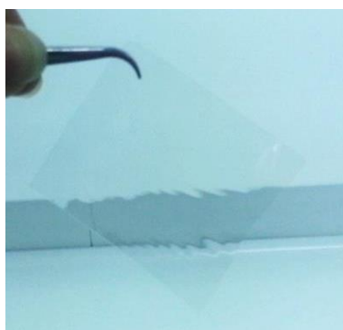
Figure 9.12. Film of PVA used as blank realized by solvent casting procedure
