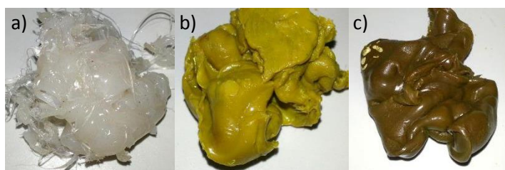
Figure 9.5. Blended matrices of PP blank (a), A1 1% (b) and A1 5% (c)
