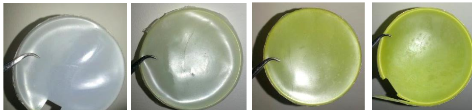
Figure 9.13. 1Dried films in Petri dishes of Mater-Bi and PEG 400 used as blank (a) and Mater-Bi and PEG 400 with 0.01%, 0.05% and 0.1% of A4 (b-c-d respectively)
