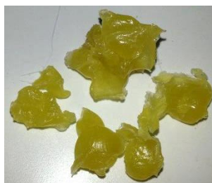
Figure 9.6. Blended matrices of PP with A1 0.01%
