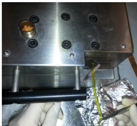
Figure 9.7. Extrusion of the matrix formed by PLA4032D and A4 0.1% using Thermo Scientific Haake Minilab II extruder
