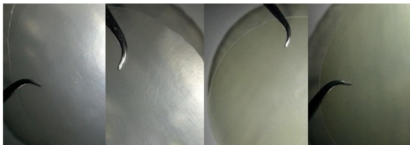
Figure 9.9. Thin film mold casted of PLA4032D blank (a); with A3 0.01% (b), A3 0.05% (c) and A3 0.1% (d)
