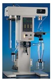
Figure 42. BÜCHI B-191 Mini Spray Dryer.
