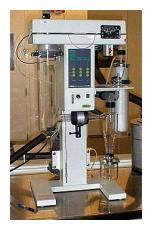
Figure 5: Mini Spray Dryer
