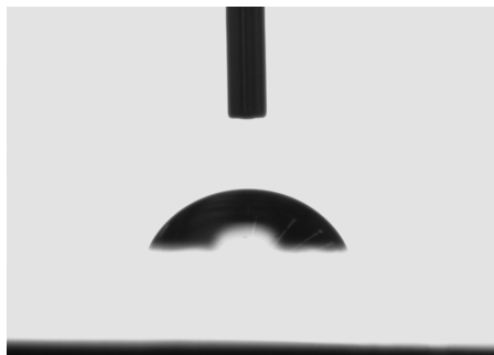
figure 6: Contact angle on a 200nm-thick cured film surface of PMMA ( 67.2^\circ ).
