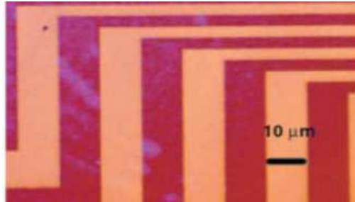
figure 10: optical imaging of micrometric structures obtained in [15] by local optical polymerization of pentacene precursor films.
