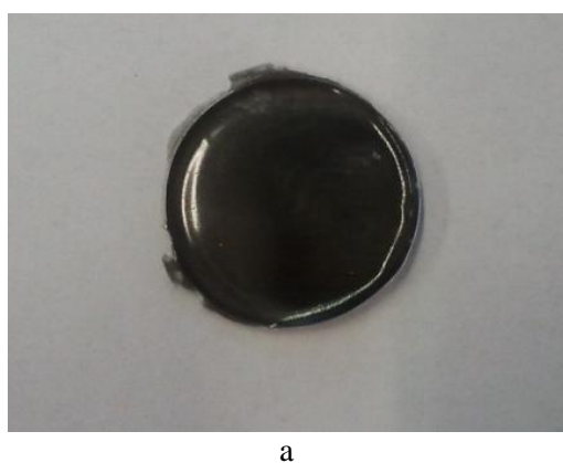
Figure V.20 CA/GO structures obtained at 200 bar 40 °C starting from 25% w/w CA/NMP solution and 3% w/w of GO: a) macroscopic view, b) FESEM analysis of the section, c) FESEM analysis of the top surface
