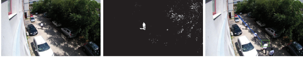
FIGURE 6.4: Illustration of the preliminary results obtained by the proposed tracker: (left) sample image acquired with the wide-view camera; (middle) foreground regions attained by background subtraction; (right) people tracking module results. The blue dots highlights the point tracked over the time.
