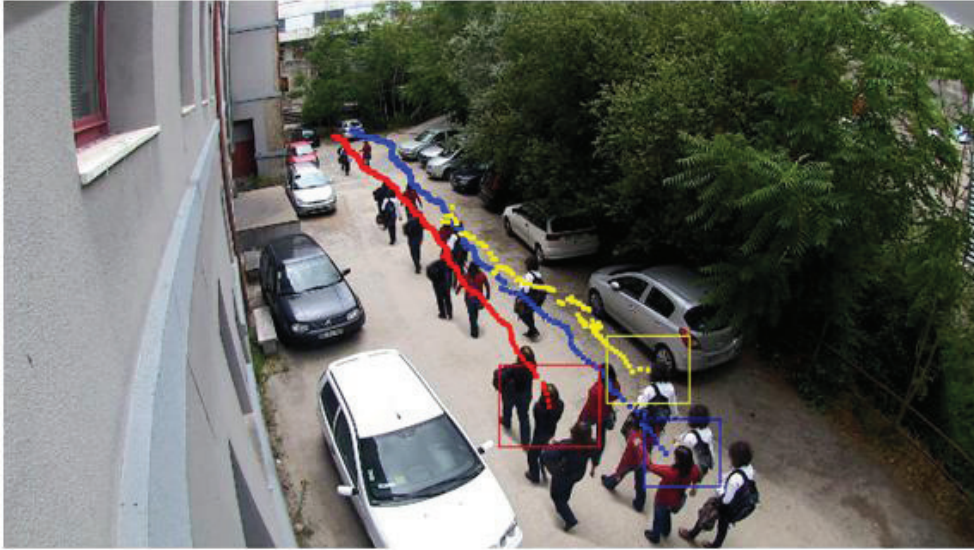
FIGURE 6.5: The image, obtained by overlapping several frames grabbed over the time in a single image, shows how the tracker is able to keep track of more than one people.
