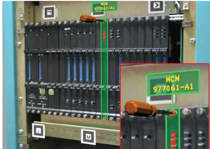
FIGURE 3.1: An example of augmenting an industrial equipment with a virtual screwdriver that suggests the screws to be unmounted during a specific step of the maintenance procedure.
