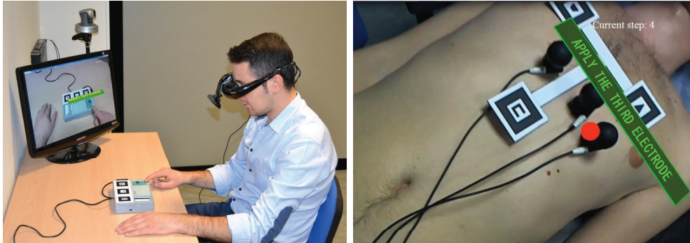
FIGURE 3.3: The possible scenarios of usage of the proposed telemedicine prototype. The user wears the HMD and observes the ECG device. From the system he/she receives visual and audio feedbacks to guide him/her during the setup (left). The thorax of a real patient augmented of virtual aids to a proper placing of the electrodes (right).
