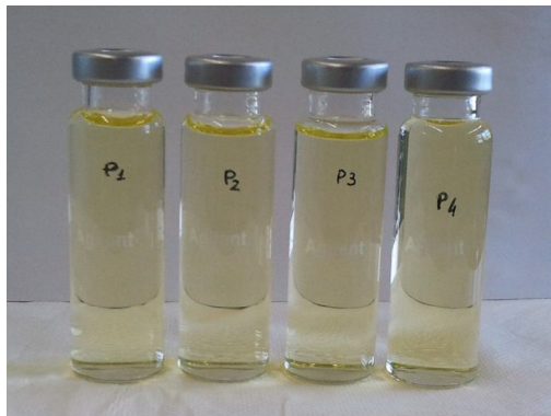
Figure XIV. 2 Macroscopic aspect of \beta -C nanoparticles suspensions produced by SAILA with variation of GLR. Process conditions are reported in Table 14.
