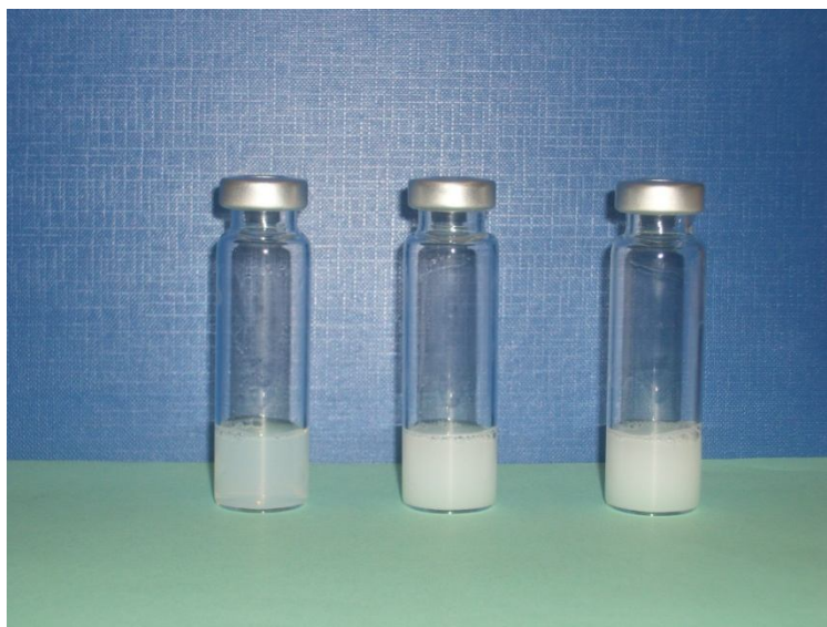
Figure XI. 5 Macroscopic aspect of nanoparticle suspensions obtained with different PCL content. The polymer percentage in solvent phase is 0.5, 1.0, 2.0 from the left to the right of the image
