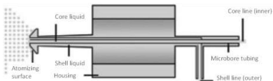
Figure 28. Dual liquid feed assembly [66]
