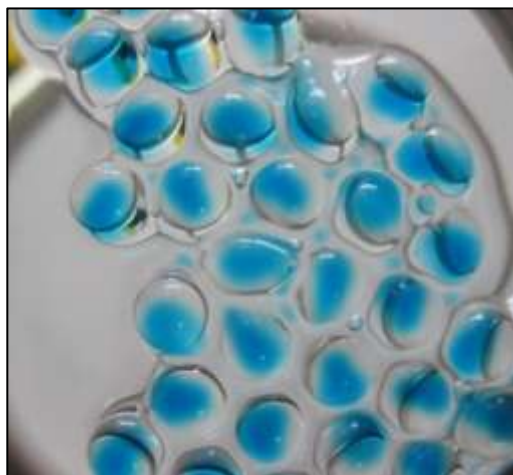
Figure 33. Example of shell-core particles: blue core confined in the transparent shell material
