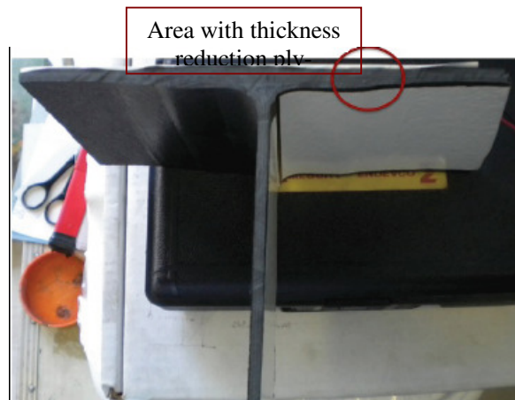
Fig. 3.14- Detail of the area with reducing thickness partially responsible for the energy concentration.
