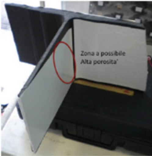
Fig. 3.17 - Detail of the area potentially concerned by high porosity
