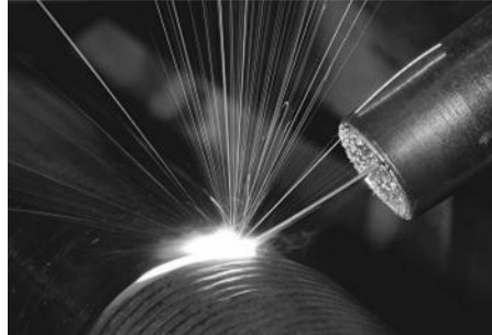
Fig.2.4 Laser Cladding by wire feeding.
