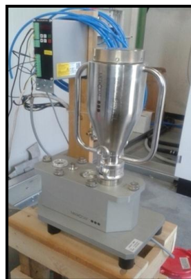
Fig.4.5: Vibrating powder system.
