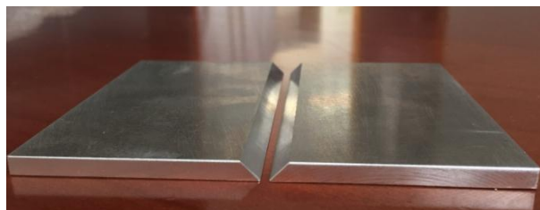
Fig. 5.16: V-groove aluminum plate.
