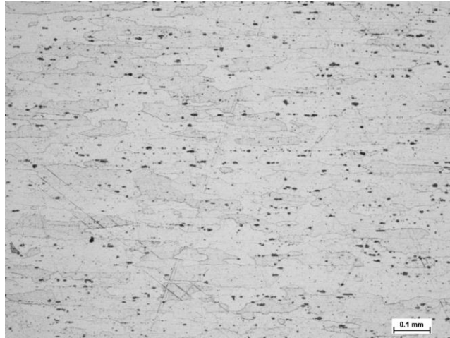
Fig. 5.30: Base material, aluminum matrix.
