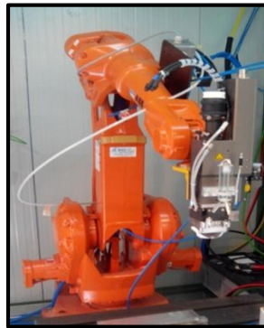
Fig.4.4: six-degree of freedom industrial robot.
