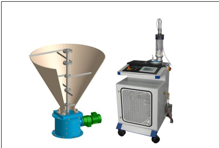
Fig.3.11: Mechanical wheel powder feeder.
