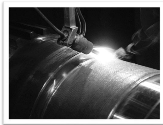
Fig. 1.3: Laser cladding repair
