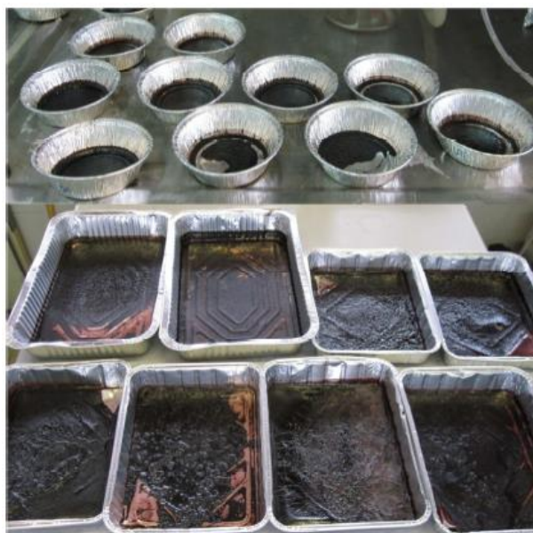
Figure 26. Dried samples extracted during synthesis reaction (on the top) and dried final product (on the bottom)
