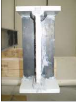
Figure 4.4a. Web-flange reinforcement – cross end view.
