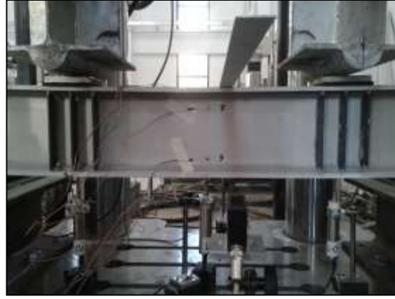
Figure 4.4b. Web-flange reinforcement – frontal view.
