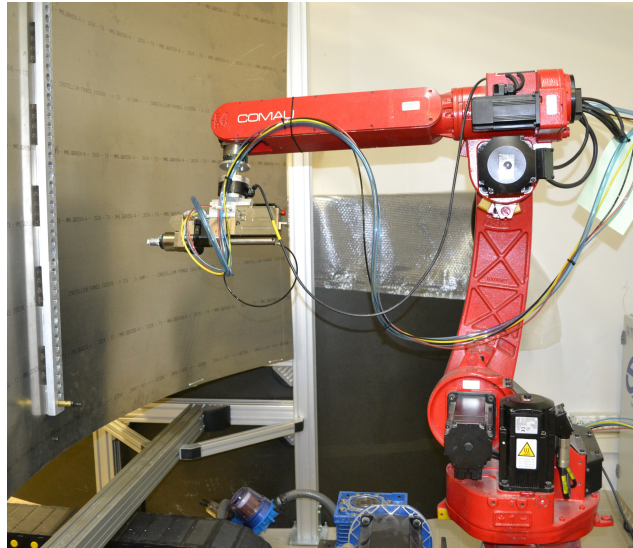
Figure 2.5 Robot with Drilling tool.
