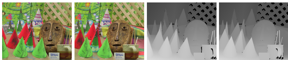
Figure 1.5: Dense stereo matching problem input (first two images) and output (last two images).
