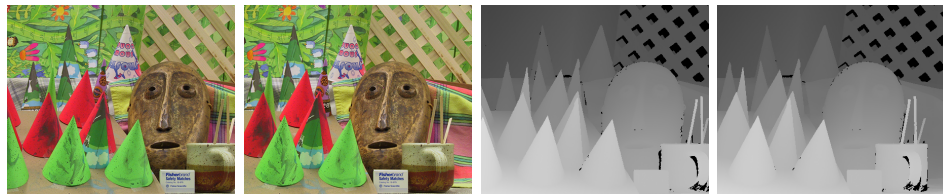
Figure 1.5: Dense stereo matching problem input (first two images) and output (last two images).
