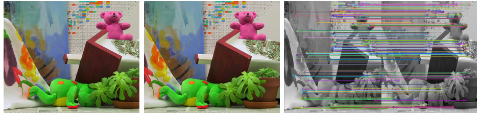
Figure 1.4: Sparse stereo matching input (first two images) and output (last image). The horizontal lines represent the few matched point on both images.
