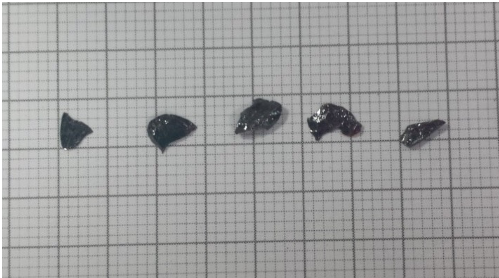
Figure 2.8: Crystal samples of \text{Cu}_3\text{Nb}_2\text{O}_8 from batch No.3
