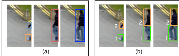
Figure 3.2 Problems with entering objects. (a) Blobs across three adjacent frames. (b) The tracking performed without considering the object history; in this case a tracking algorithm would not be able to distinguish this situation from two separate objects joining a group, and so attempts to preserve the separate identities of the two objects 1 and 2.
