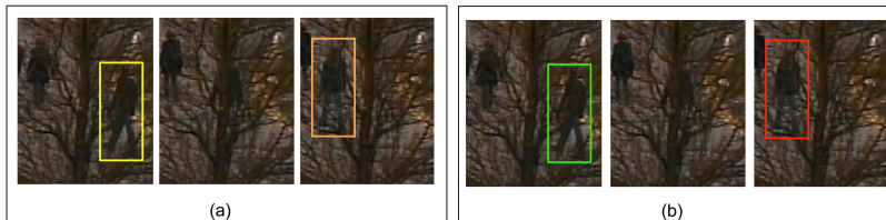
Figure 3.3 Problems with totally occluded objects. (a) The detection output across three adjacent frames. (b) The tracking performed without considering the object history; in this case a tracking algorithm would see the blob 2 as a new object in the scene, since in the previous frame there was no corresponding object.
