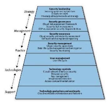
Figure 1.2: An enterprise security architecture for Cloud Computing.
