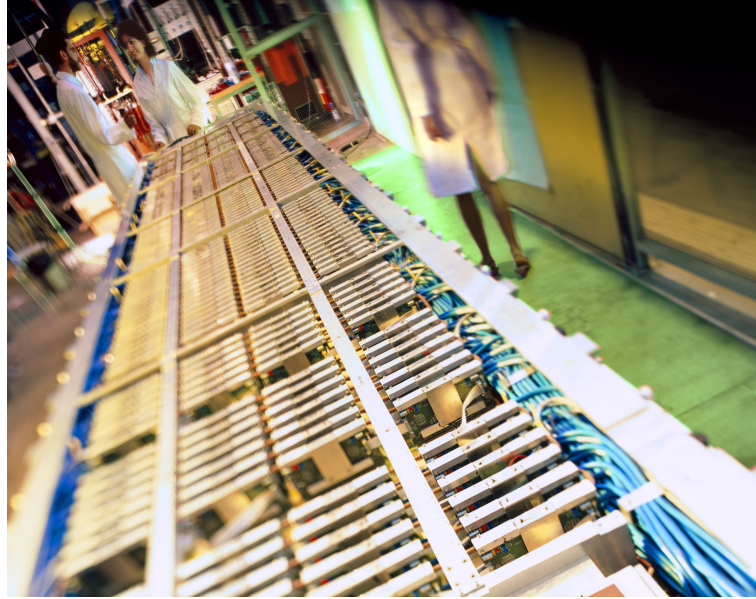
FIGURE 4.3: A supermodule of the TOF detector after assembly.
