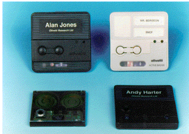
Figure 2.1 Active Badge modules: bottom left, the first version, with a unique five bit code; bottom right, the second version, with a ten bit code; top left, the third, current, version, with a forty-eight bit code, bi-directional capabilities, and an on-board 87C751 microprocessor. Source: http://www.cl.cam.ac.uk .
