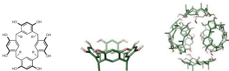
Figure 32. Left, chemical structure of resorcin[4]arene; middle, representation of the same resorcin[4]arene; right, representation of the hexameric resorcin[4]arene capsule.
