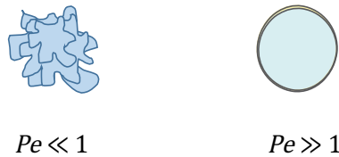
Figure 17. Proposed particle formation during the spray drying process: for a low Peclet number, corrugated microparticles will be formed; for a high Peclet number, a shell with a spherical shape will be formed.
