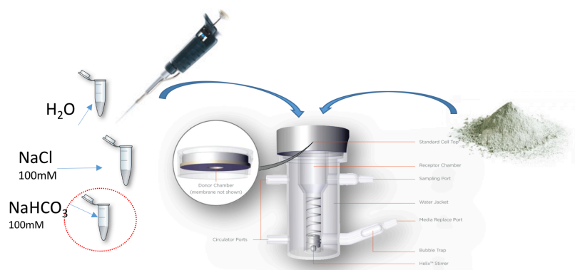
Figure 18. Schematic representation of the dissolution process of KLys after the pre-treatment of the CF sputum samples and the addition of the powders, respectively, to the donor compartment of a vertical diffusion cell (Franz cell apparatus).
