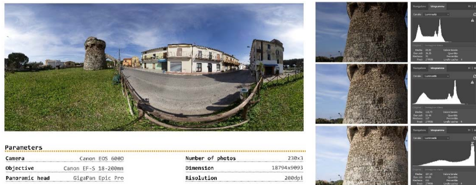
Figure 3.11: Parameters of panoramic taken with Canon EOS 600D and HDR acquisition
