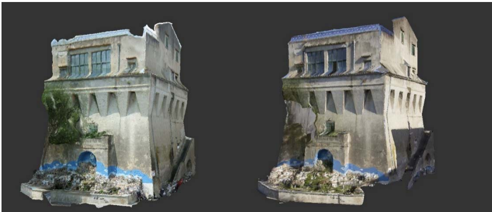
Figure 6.7: ReCap Photo models with photos taken from Fujifilm XF1 and Canon EOS 600D
