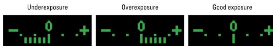
Figure 4.25: The bars under the meter indicate the amount of under or overexposure
