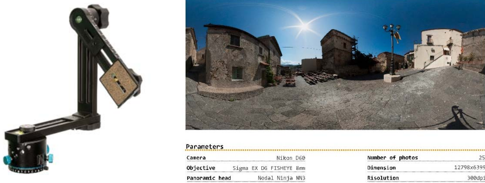
Figure 3.12: Panoramic head NN4 and parameters of panoramic photo with Nikon D60
