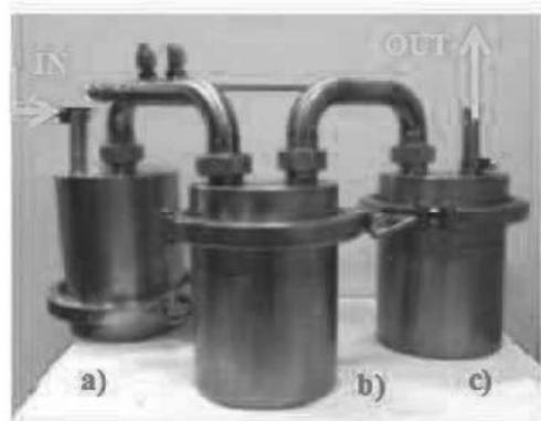
**Figure VI.9:** *Second stage of sulphur abatement (a) and water condenser with pollutants removal (b,c).*
