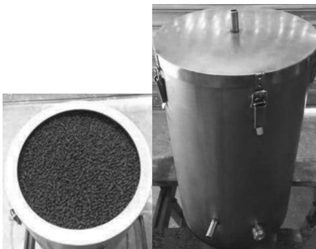
**Figure VI.10:** Activated carbon for  $H_2S$  residual removal by adsorption.
