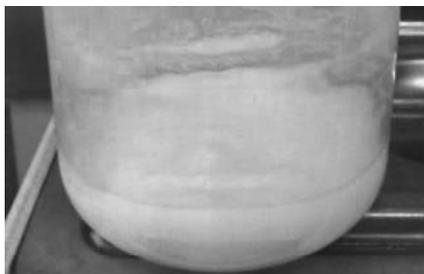
**Figure X.1:** *Monolith dipped in the washcoat.*
