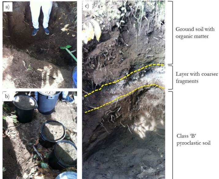
Figure 5.10 The material collected in Tuostolo Basin: a) excavation; b) pots for the transporting the material collected and c) observed stratigraphic setting of the excavation.
