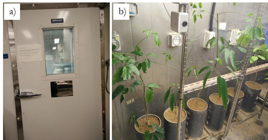
Figure 4.7 a) Environment controlled room placed inside the Geotechnical laboratory of HKUST and b) vegetated columns.
