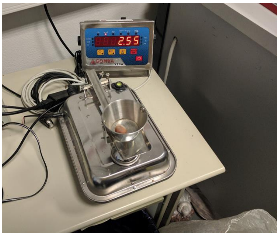
Figure IV-7 Scale with a 0.05 g resolution
