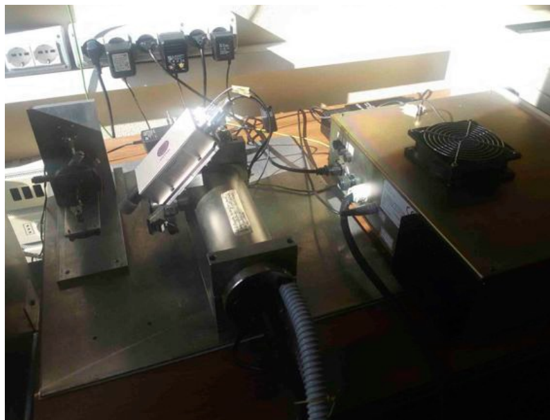
Fig. 5.2.: Picture of XRF set up used for archaeometric analysis
