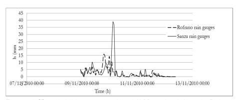
Figure 7.3: The rainfall hyetographs of the 9-11 November 2010 at the Rofrano and Sanza rain gauges.
