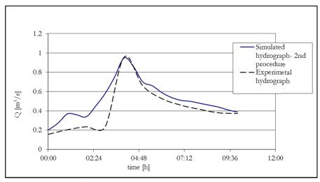
Figure 7.8: The hydrograph simulated with the second procedure is compared to the experimental one.
