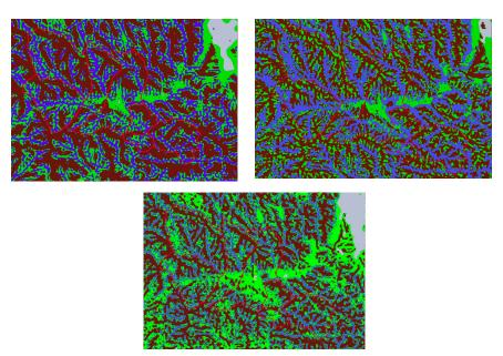
Figure 5.16: The three TPI maps, performed in the test-region, chosen for calculate the Fragmentation Index. On the upper left 5 - 25 coupled, on the upper right there is the coupled 6-36 and on the bottom center the coupled 3-9
