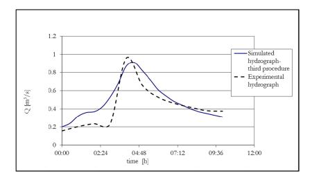
Figure 7.9: Comparison between the simulated and experimental hydrograph
