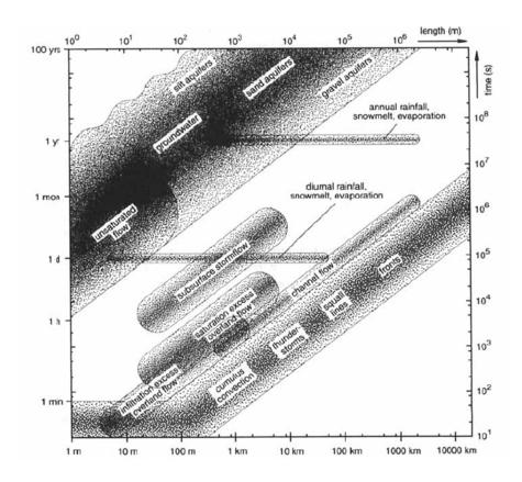
Figure 2.4: Hydrological processes at a range of characteristic space time scales (from Blosch and Silvapan, 1995).
