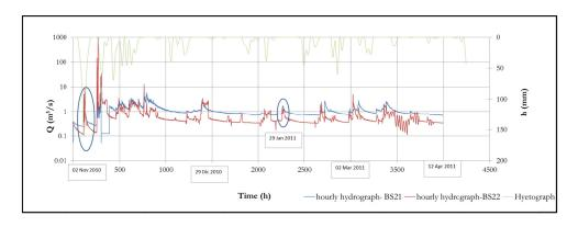
Figure 6.26. Hydrograph of the catchments BS21 and BS22 detected from October 2010 to April 2011. The blue line evidence the two event storms analyzed
