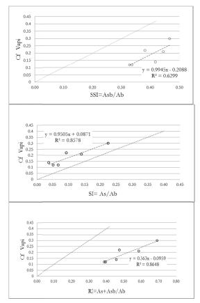
Figure 6.28: Straight line equation between the SSI and Cf, SI and Cf, RI and Cf
