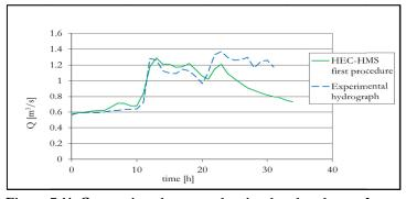
Figure 7.11: Comparison between the simulated and experimental hydrographs.
