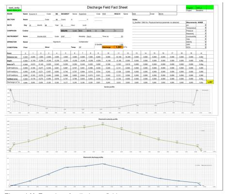
Figure 4.38: Fact sheet for discharge field measurements.
