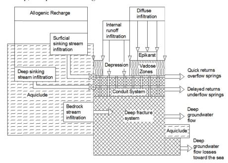
Figure 4.27: Conceptual model of Bussento Hydrogeological System (BHS) (modified from Guida at al., 2003)
