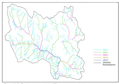
Figure 3.18: Drainage network and Horton stream ordering.
