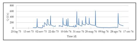
Figure 6.37: The hydrograph of the Torna catchments detected from 1 october 1975 to 27 september 1976
