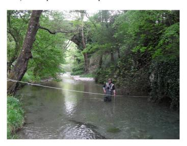
Figure 4.37: Direct discharge measurements with Swoffer 3000.
