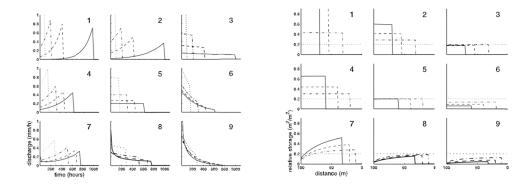
Figure 6.9: The hydrological behavior of the nine Basic geomorphometric Types (BGT):on the left, the sub-surface flow rate at different location along the hillslope; on the right, soil moisture storage for characteristics time steps during the free drainage (Troch et al., 2002)
