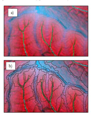
Figure 6.14: a) the map is a composed of the DEM, slope, planar and profile curvature, and flow accumulation (grid image); b) the results map of the segmentation algorithm is shown (object image)
