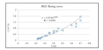
Figure 4.42: Rating curve of the BS21 river section
