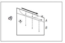
Figure 6.20: The Hortonian Overland Flow (HOF) is considered for conditions: on the left infiltratin restricted by a low permeability layer in the A or upper B horizon caused by compaction; on the right on nearly saturated shallow soils, infiltration quickly causes saturations (modified from Scherrer et al., 2007)
