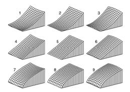
Figure 6.6: The nine form element, corresponding to Basic Geomorphometric Types (BGT): 1. Concave in plan and in profile; 2. Straight in plan and convex in profile; 3. Concave in plan and convex in profile; 4. Convex in plan and straight in profile; 5. Straight in plan and profile; 6. Concave in plan and straight in profile; 7. Convex in plan and concave in profile; 8staight in plan and concave in profile; 9. Convex in plan and in profile.
