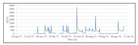
Figure 6.35: The hydrograph of the Nocellito catchments detected from 1 october 1975 to 27 september 1976
