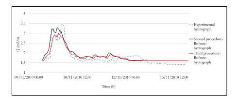
Figure 7.14: The comparison between the hydrographs simulated with the second and third procedure and the experimental one. In the simulations was used rainfall of the Rofrano station.
