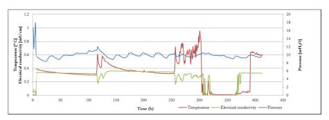
Figure 4.40: Integrate measurement plots (Water Level, Temperature and Electrical Conductivity) at BS21 (Inferno Bridge) station during the November 2010 Flood Event. Note the no-registration due to instrument damage (fig. 4.41).
