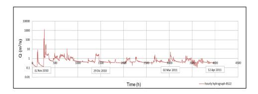
Figure 4.44: Hydrograph performed with hourly stream flow data colleted at the BS22 river station.
