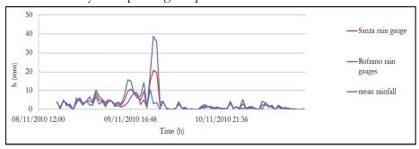
Figure 7.12: The hyetograph of the rainfall measured at the Rofrano and Sanza rain gauges
