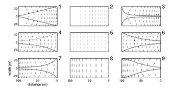
Figure 6.8: Plan view of drainage devides (solid lines) and contour lines (dashed lines of nine BGTs. The upslope devide is at x=0 (Troch et al., 2002)
