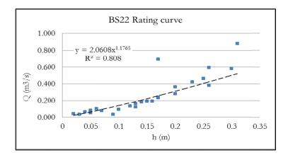
Figure 4.43: Rating curve of the BS22 river section
