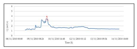
Figure 7.10 The observed hydrograph for the event of the 9-11 november 2010. The line in red indicate the effective water level.
