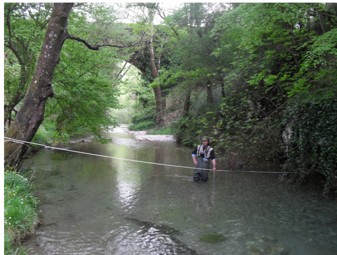
Figure 4.37: Direct discharge measurements with Swoffer 3000.
