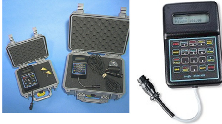
Figure 4.36: Current meter Swoffer 3000
