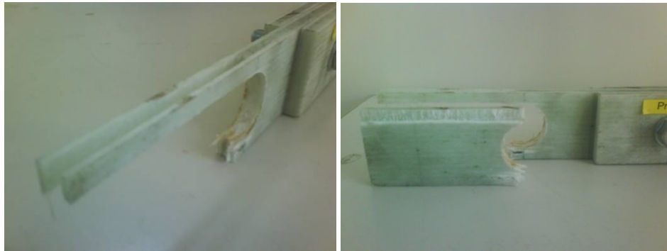
Figure 4.11. Joint J21 failure.
