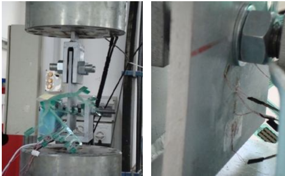
Figure 6.2. GFRP specimens in the machine test.
