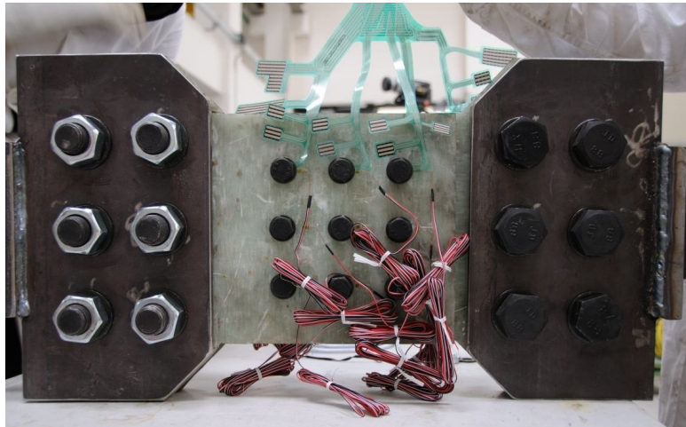
Figure 4.47. Joint J33 Type 2, assembled and instrumented.
