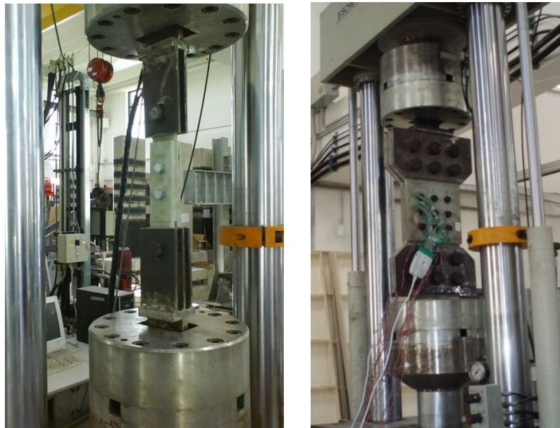
Figure 4.1. Universal machine SCHENCK Hydropolus S56.
