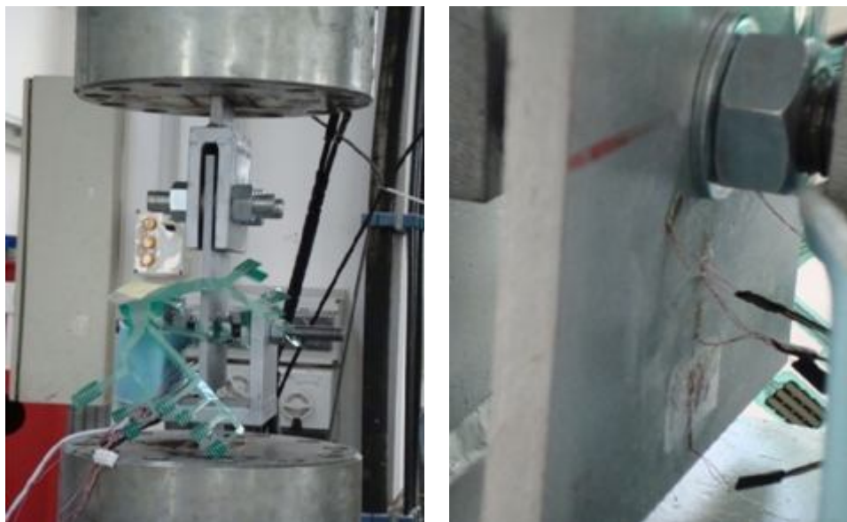
Figure 6.2. GFRP specimens in the machine test.
