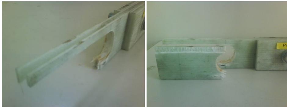
Figure 4.11. Joint J21 failure.
