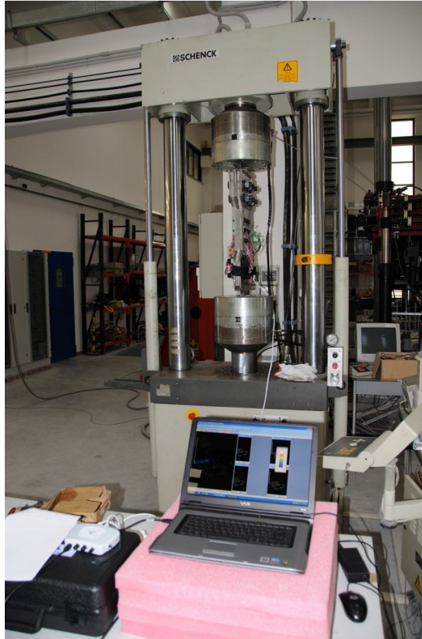
Figure 4.49. Joint J33 Type 2 in the test machine.
