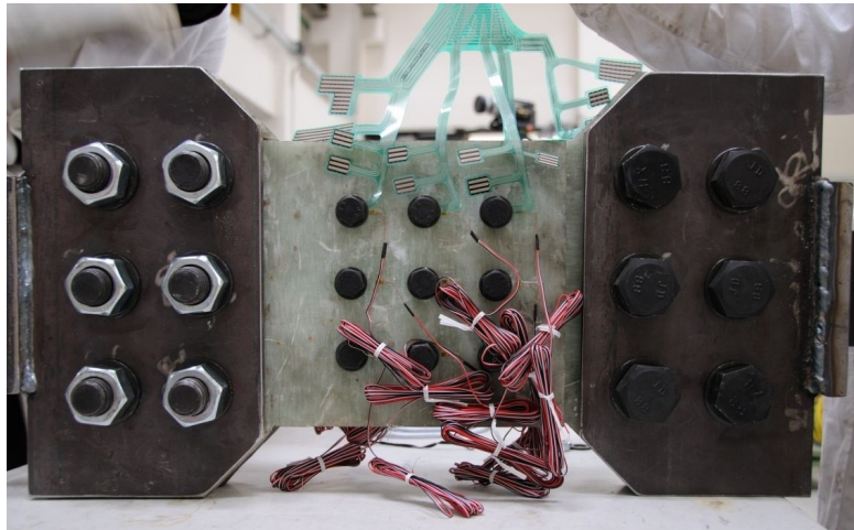
Figure 4.47. Joint J33 Type 2, assembled and instrumented.
