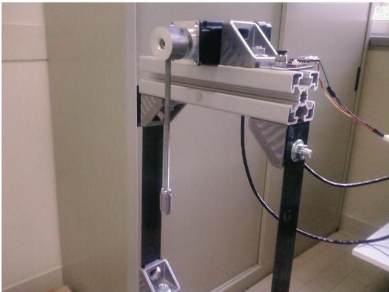
The control actuator is realized by a simple pendulum which can oscillate along the plane of the structure. The pendulum is driven by a Kollmorgen AKM brushless motor, equipped with an encoder, which provides the control torque.
