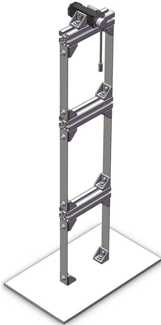
The length of the structural elements are equal respectively to  $L_1 = 23 \cdot 10^{-2} [m]$ ,  $L_2 = 28 \cdot 10^{-2} [m]$  and  $L_3 = 23 \cdot 10^{-2} [m]$  whereas the half-length of the pendulum is equal to  $L_4 = 8.25 \cdot 10^{-2} [m]$ . The dimensions of the cross sections relative to the structural elements are  $b_1 = b_2 = b_3 = 3.5 \cdot 10^{-2} [m]$
