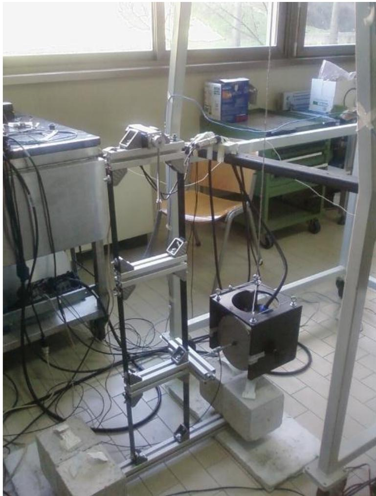
The frequency range of interest encompasses all the frequencies below  $15 [Hz]$ . In the frequency range of interest, the steel beams behave like flexible
