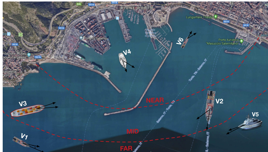
Figure 7.12 Position and drifting angles of the six vessels of the case study.
