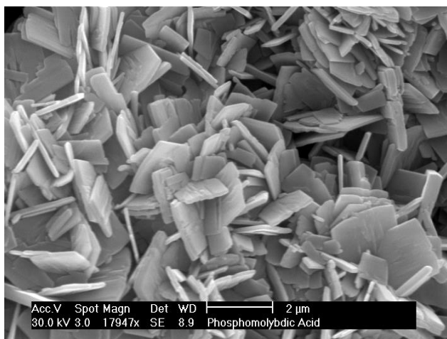
Figure 5.8. Environmental Scanning Electron Microscopy (ESEM) of crystals of H_3PMo_{12}O_{40}
