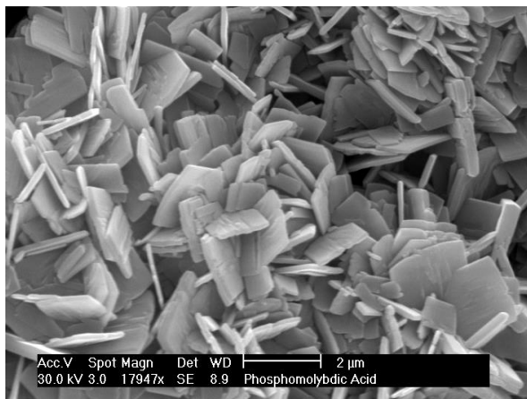
Figure 4.6. SEM image of \text{H}_3\text{PMo}_{12}\text{O}_{40} Nanoparticles
