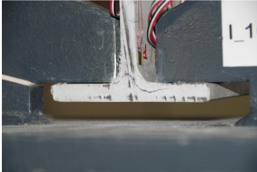
Figure 3.10. Web/Flange Junction Failure of I_160_EP_3 specimen.
