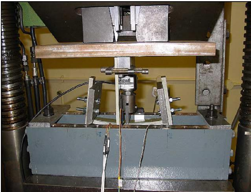
Fig. 1.62. Photograph showing the dual knife-edges loosely clamped to the upper half-flange at each end of the WF specimen.
