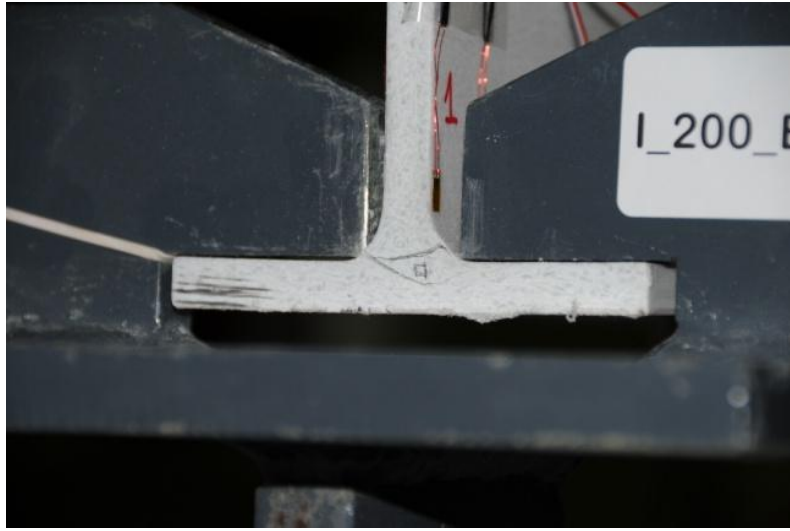
Figure 3.23. Web/Flange Junction Failure of I_200_EP_2 specimen.
