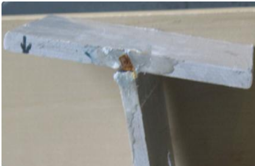
Figure 4.40. Failure of H 6" × 6" × 3/8" (152.4 mm × 152.4 mm × 9.53 mm) R specimen.
