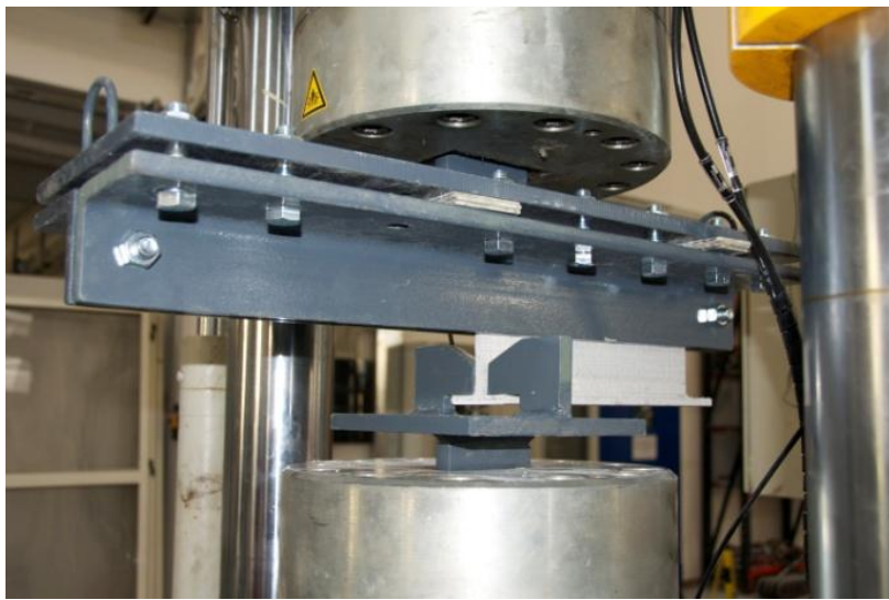
Figure 3.1. End Point Pull-Out Test Setup.
