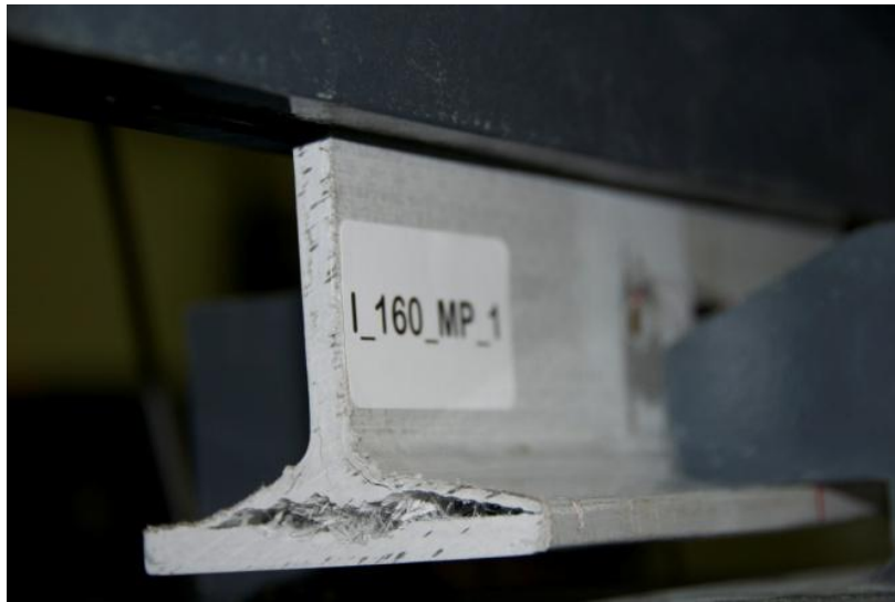
Figure 3.16. Web/Flange Junction Failure of I_160_MP_1 specimen.
