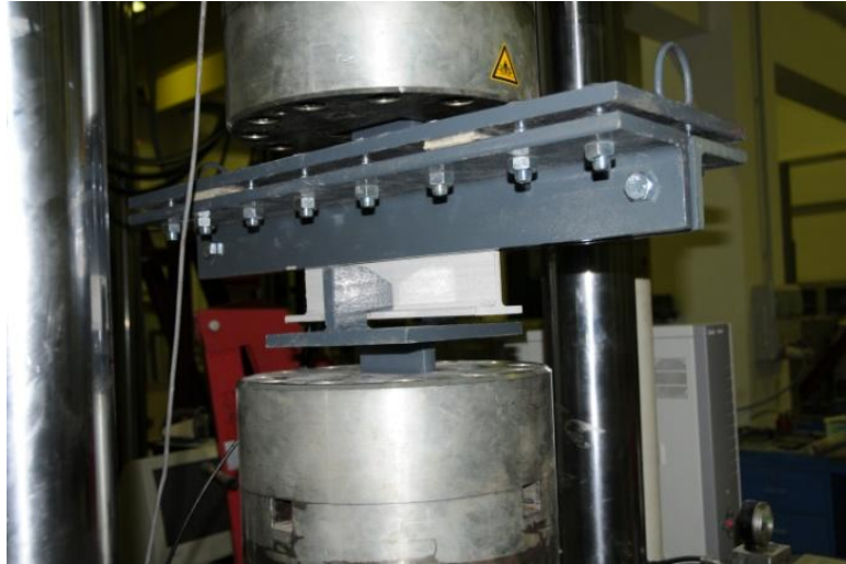
Figure 3.2. Mid Point Pull-Out Test Setup.
