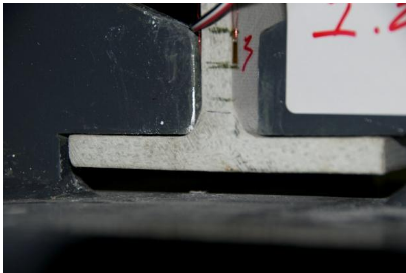
Figure 3.27. Web/Flange Junction Failure of L_200_EP_4 specimen.
