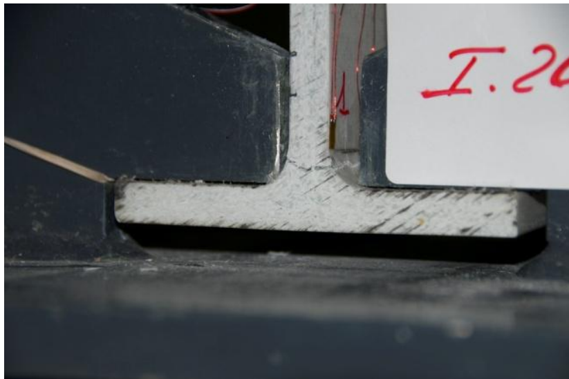
Figure 3.26. Web/Flange Junction Failure of I_200_EP_3 specimen.
