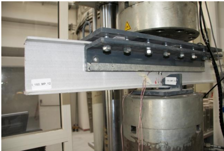
Figure 3.35d. Failure mode of I_160_MP_12 specimen of 1200 mm length.
