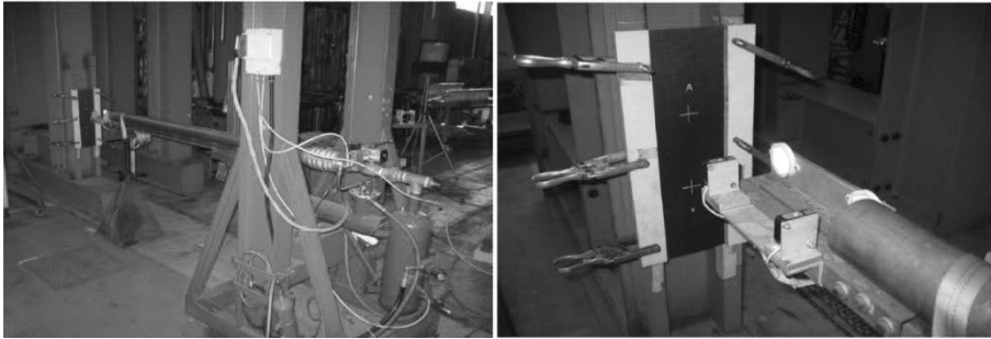
Figure I.17 Hail Impact Test set up (on the left) and Test fixture (on the right)
