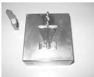
Figure III.7 Metallic mould for sample preparation
