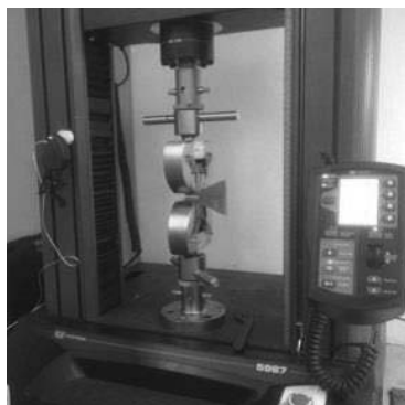
Figure II.8 Equipment to evaluate the healing efficiency
