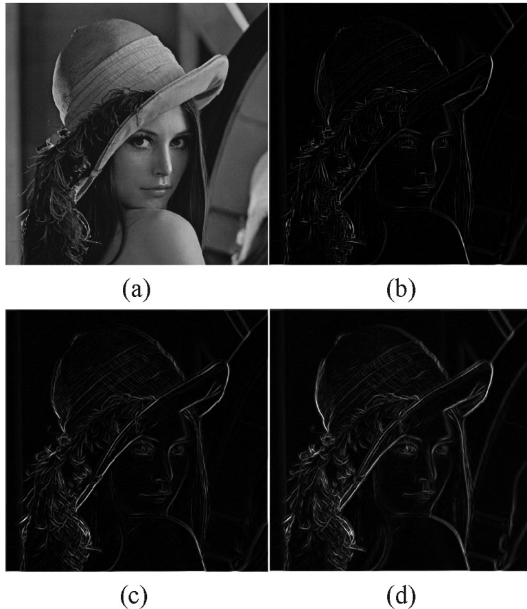
Figure IV.4 (a) Original Lena image and obtained results for f_0 = 0.2 , \gamma = 1 , \eta = 15 considering 7 \times 7 Gabor filter and (b) two, (c) four and (d) eight orientations.
