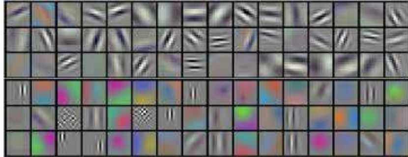
Figure V.5 The 96 kernels used for the processing of the first convolutional layer in AlexNet
