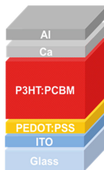
Figure 5.1 Sketch of the cross-section of the investigated polymer:fullerene solar cells.
