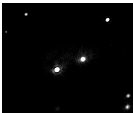
Figure IV.5 Example of frame from NTA analysis of liposome suspensions produced at a PC concentration of 5 mg/mL and 1% fluorescein theoretical loading.
