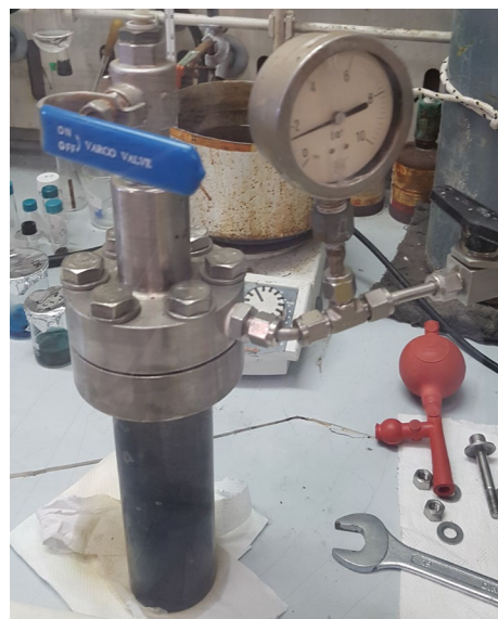
Figure 10 - Autoclave for hydrothermal synthesis of GO-ZnO
