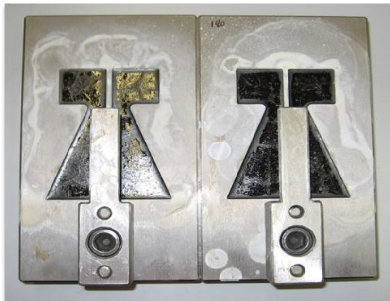
Figure 115: Cured Self-healing Samples before extraction from the molds
