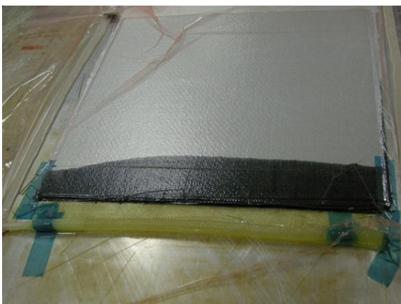
Figure 130: Moment of Fiber Impregnation
