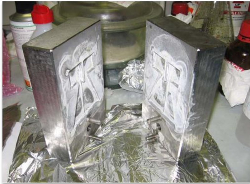
Figure 114 Metallic Molds (with teflon sprayed) for self-healing specimens with TDCB geometry
