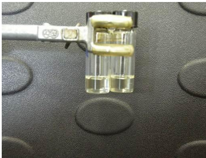
Figure 100: ENB/ 2.5% DCPD and ENB/ 5%DCPD blends after 1h at -50 °C
