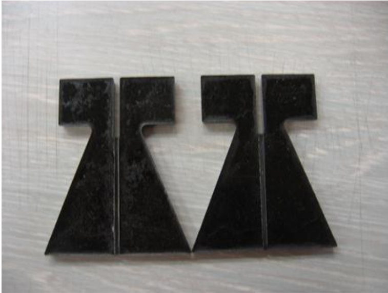
Figure 116: Cured Self-healing samples after extraction from metallic molds
