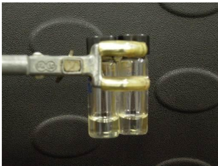
Figure 101: ENB/ 2.5% DCPD and ENB/ 5%DCPD blends after 5h at -50 °C
