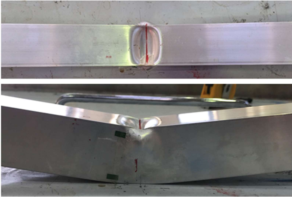
Figure 3.21. Close-up of beam after testing showing typical formation of local buckles.
