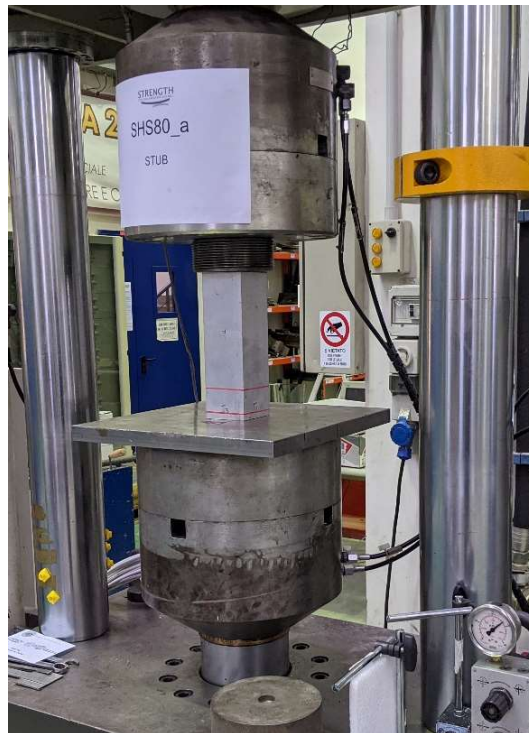
Figure 3.9. Setup of stub column test.
