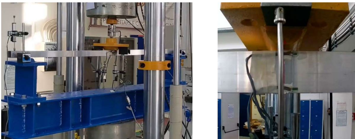
Figure 3.16. Setup of Three Point Bending Test.
