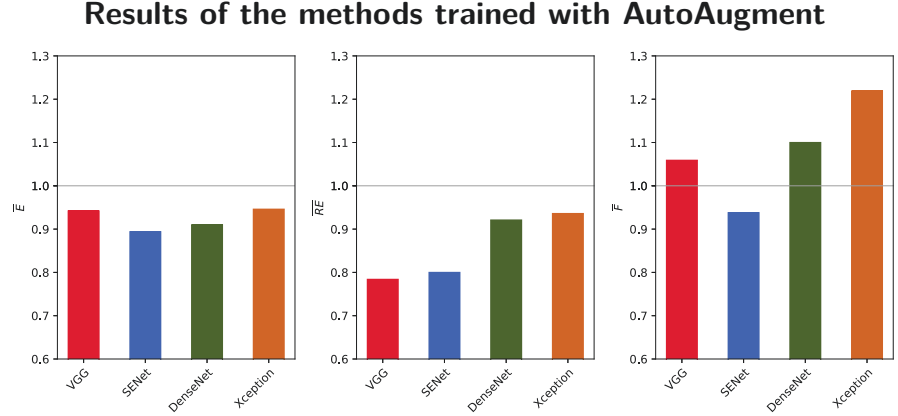
Figure 4.3: Results achieved by the considered methods trained with AutoAugment. For each method, the mean error \bar{E} (left plot), the relative error \overline{RE} (middle plot) and the flip rate \bar{F} (right plot) are computed using the corresponding method without AutoAugment as the baseline, represented as the 1.0 horizontal line.
