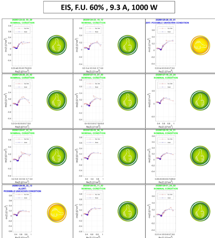
Figure 3.30: On-field test n.2 - On-board algorithm outcomes for F.U. 60% - Nominal Condition. The spectrum is acquired via conventional stimuli. Here the yellow thumbs indicates a possible unknown condition. This occurrence can be due either to a false alarm or a condition in which the diagnostic features extracted are on the edge of the defined thresholds. In this case some of the relevant symptoms are activated (i.e., value "1") whereas others are still "0". It usually happens when the FC is slowly moving towards the malfunctioning, due to an increasing drift of the relevant parameters from the nominal conditions.
