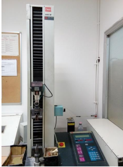
Figure 47: Image of dynamometer used for determining wet and dry tensile and elongation of the paper.
