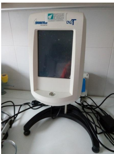
Figure 48: Image of the viscometer Brookfield DV2T used for viscosity measurement.
