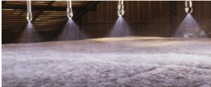
Figure 43: Binder spraying on the surface of the tape.
