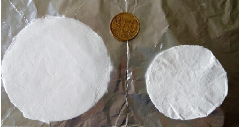
Figure 23: Shrinkage of the electrospun scaffold after the cross-linking reaction (NHS and EDC·HCl = 45.0 mM in 85.5% ethanolic solution, RT, overnight).
