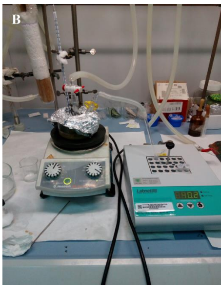
Figure 49: Photographs of the apparatus used to determine the gaseous formaldehyde released from the cross-linking: (A) without, (B) with the simultaneous reaction with acetylacetone.
