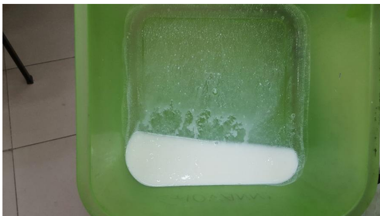
Figure 59: Image of the blend composed of XBS Binder HCHO free and PAE, with the deposited particles.
