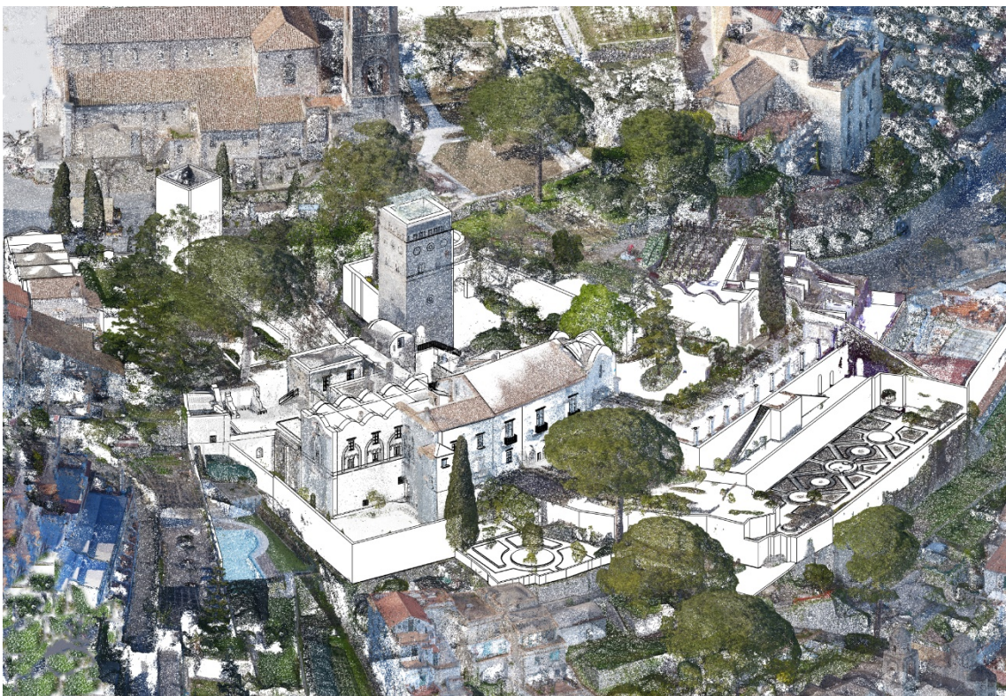
Fig. 76. Scan-to-BIM of Villa Rufolo, integrated point cloud and parametric model.
