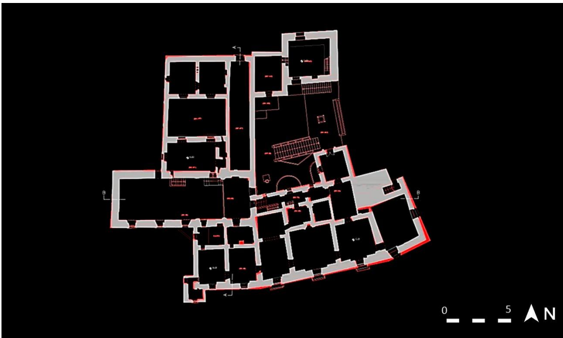
Fig. 65. Comparison between Villa Rufolo plan of 2008, in red, and plan of 2019, in grey.
