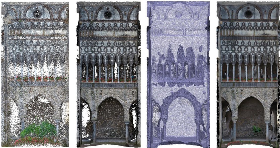
Fig. 48. Point clouds, polygonal model, and orthoimage of Chostro Moresco of Villa Rufolo.
