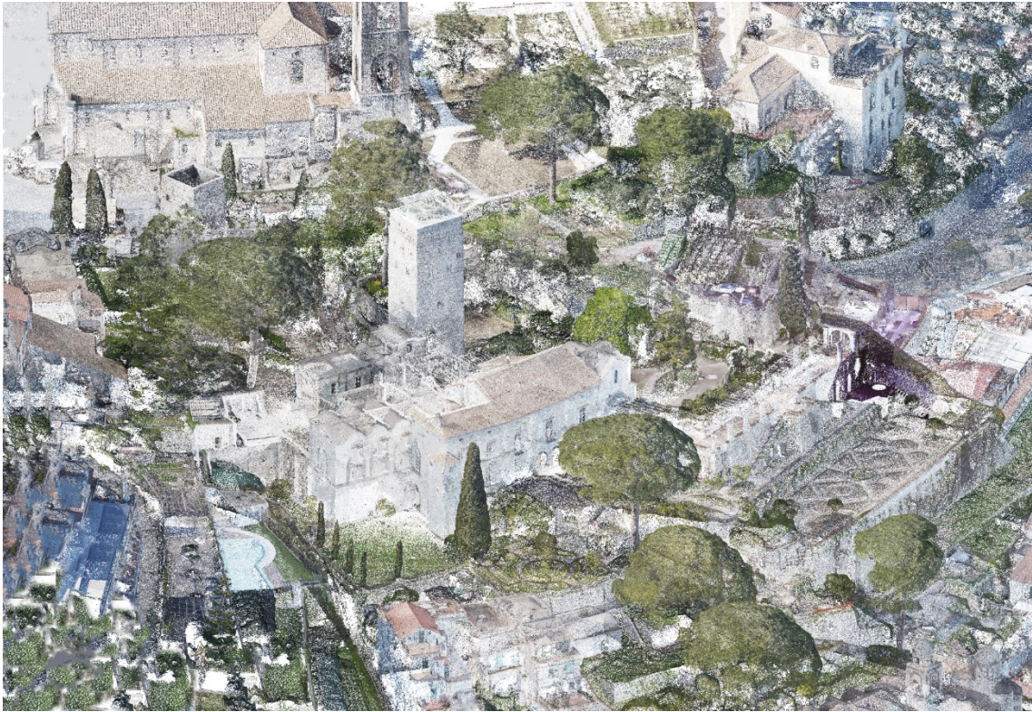
Fig. 75. Scan-to-BIM of Villa Rufolo, the integrated point cloud as basis of modeling.
