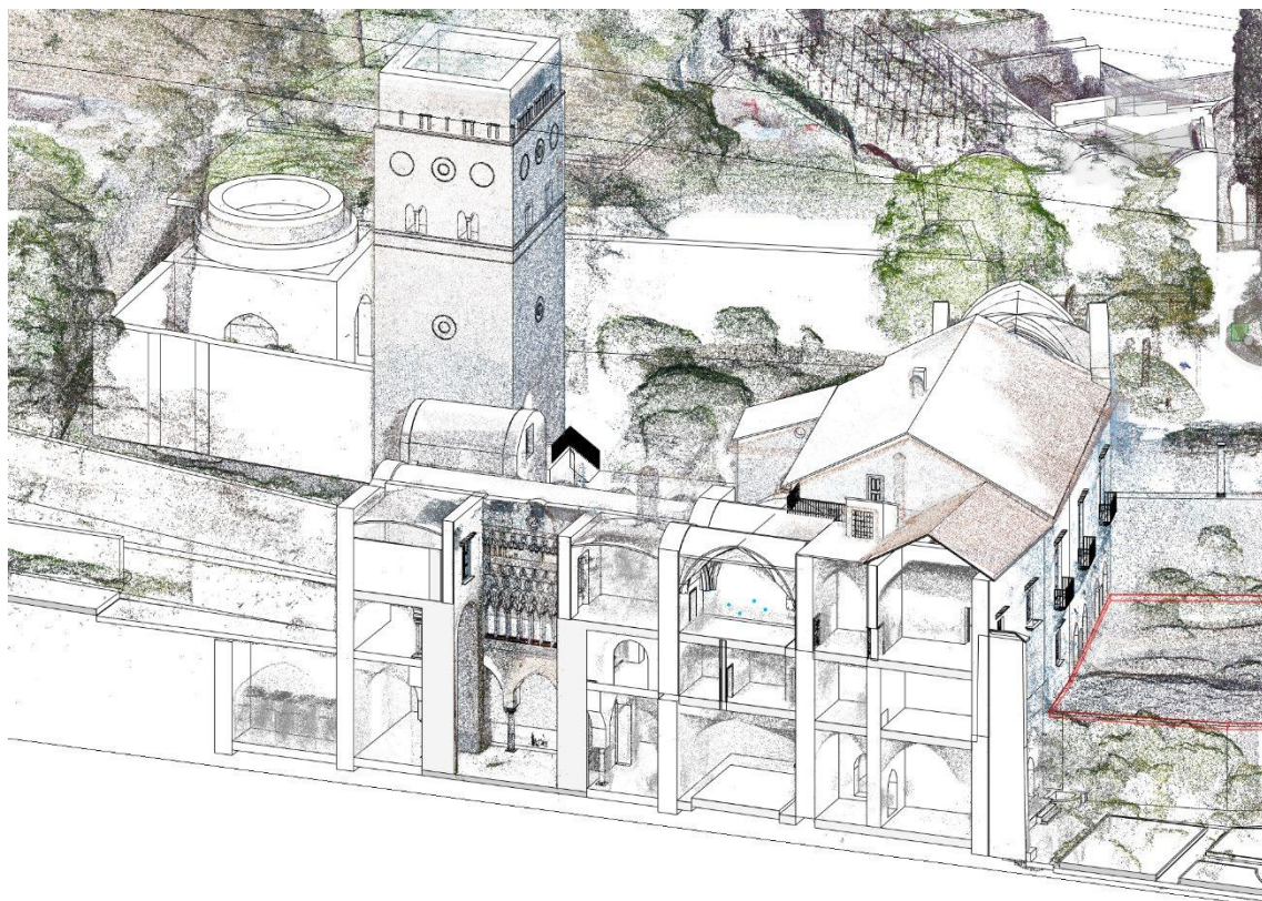
Fig. 80. Section of HBIM model of Villa Rufolo with integrated point cloud.
