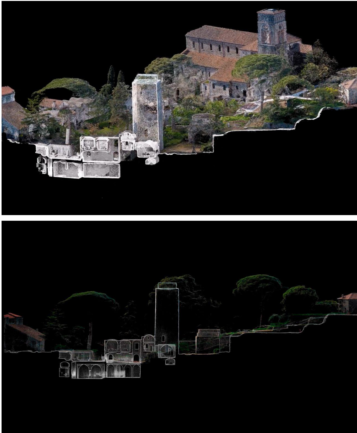
Fig. 66. Point cloud and section of Villa Rufolo.
