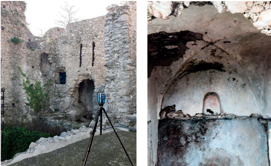
Fig. 34. The Faro Focus 3D x330 in the Balnea of Villa Rufolo in Ravello.
