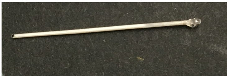
Figure 5.3. Sealed capillary used for in situ synchrotron measurements.
