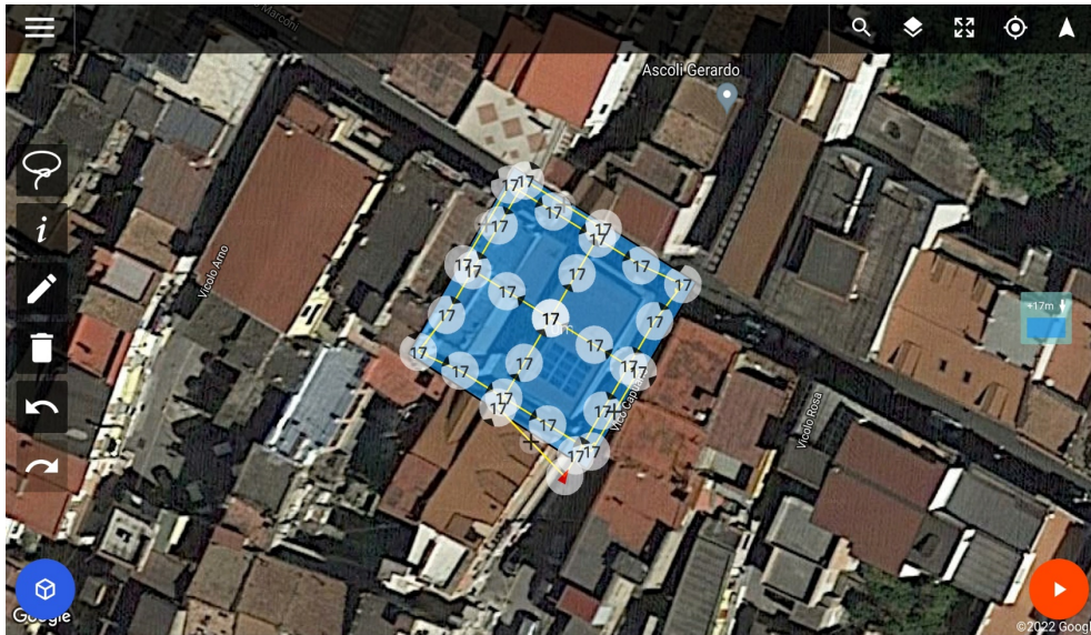
Fig. 2. 10. Flight plan map with double grid and flight height for nadiral frames.
