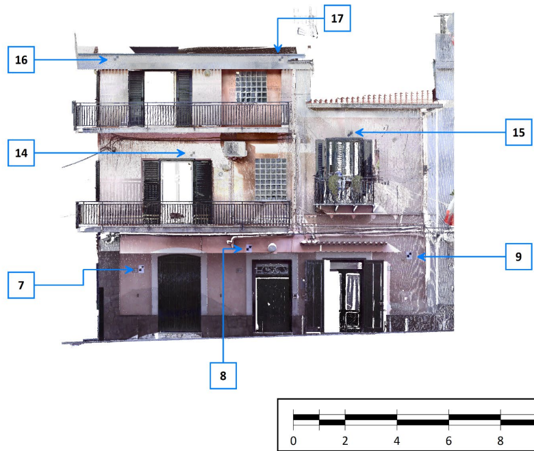
Fig. 2. 7. Checkerboard target distribution on the South-Eastern and North-Eastern facades.
