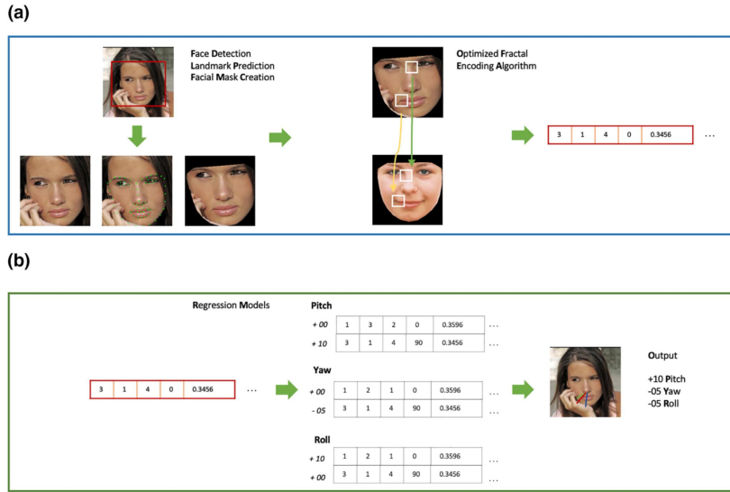
Figure 2.16: The FASHE Regression workflow: a) FASHE approach; b) GBR and XGBoost regression models.
